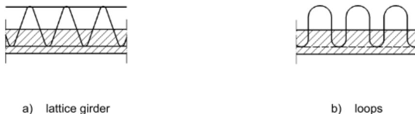
Figure 2.17 – Connecting reinforcement types [11]
