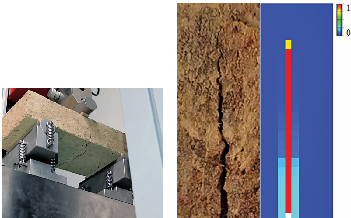
FIGURE 16. Experimental crack and numerical damage localized in the middle of a brick subjected to bending test using the adobe delta damage model in [26], a finite element model for the simulation of adobe bricks at various loading conditions and rates.
