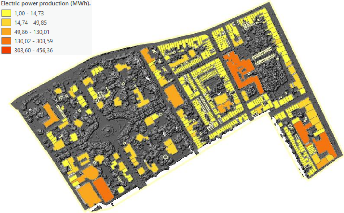
Appendix fig. A.7. Potential electricity produced aggregated per suitable building of Willemspark.
