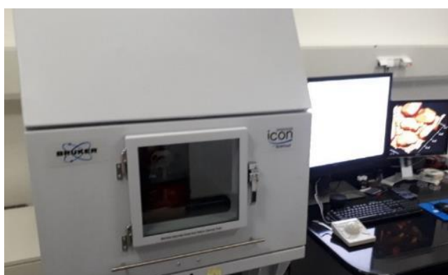
Figure S5.3. Bruker, Atomic Force Microscope with Dimension Icon ScanAsyst.
