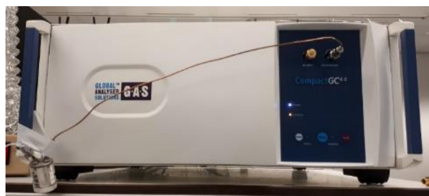
Figure S3.9. Global Analyser Solutions, CompactGC 4.0 gas chromatograph.
