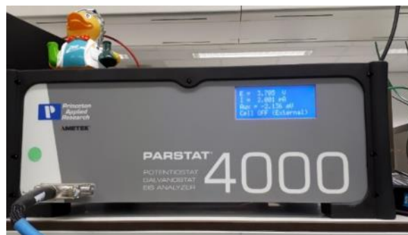
Figure S8. Ametek, Princeton Applied Research, ParStat 4000 Potentiostat /Galvanostat/EIS analyser.
