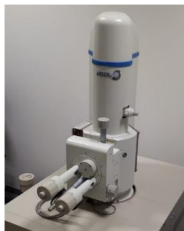
Figure S3.4. JEOL, JSM-6010LA Scanning electron microscope.
