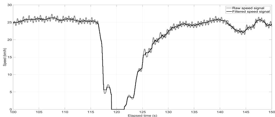
Figure 5: Filtering of the bicycle speed signal.
