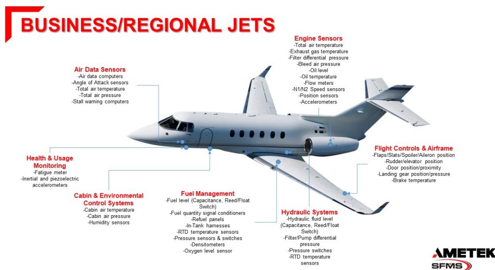
Figure 15.3: Distribution of sensors on a general business jet aircraft 9
