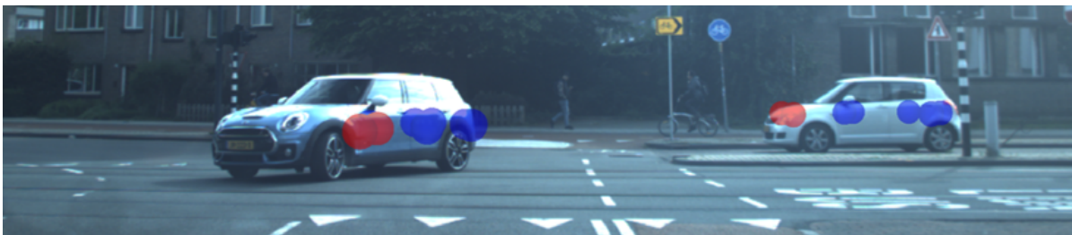
Figure 4.18: The cars that are moving slowly in lateral direction are predicted as bikers. Red dot means bikers and blue dot means car.
