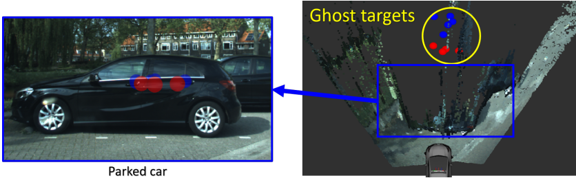
Figure 4.20: The ghost targets caused by the reflection of the ego-vehicle when there is a parked vehicle in front of it. Red dot means biker and blue dot means car.
