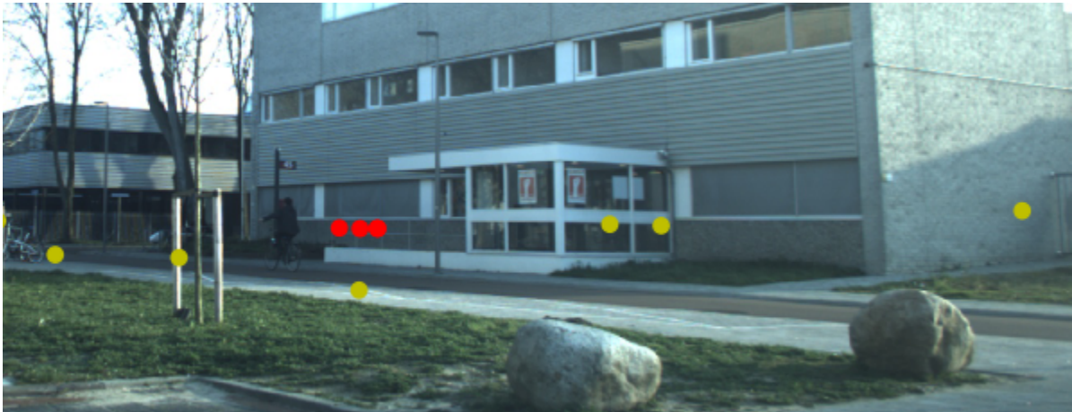
Figure 5.1: The offset between camera image and radar targets. The red targets are from the cyclist moving in lateral direction. The frame rate of camera image is only 10 Hz, less than the frame rate of radar high-level data, which is 13 Hz. When the biker is moving quickly, there will be a mismatch between camera image and targets.
