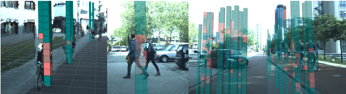
Figure 4.14: The Doppler signature visualization of different road users. Each 3D cube represents the Doppler responses at that position at a certain speed bin. The block on the ground plane represents the speed bin corresponding to the measured speed of that target.
