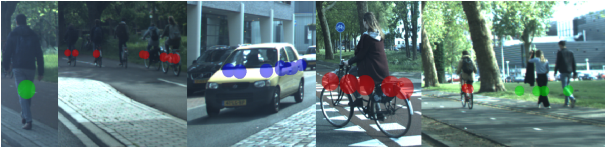
Figure 4.15: Targets predicted as road users are projected to 2D image. Green is used for pedestrian. Red is used for cyclist and blue is used for cars.
