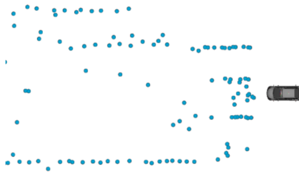
Figure 2.11: This figure shows the target list of a single radar frame from the top-down view. The vehicle is heading towards the left. The blue points are radar targets.
