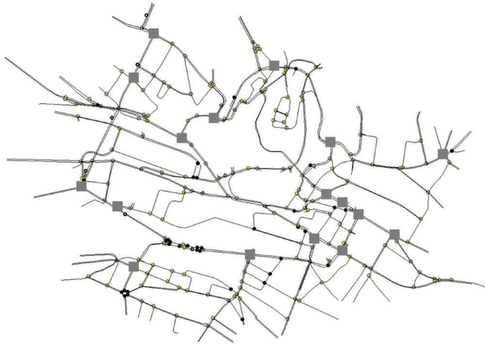
Figure 7. (Color online) Lausanne Network Model with the 17 Controlled Intersections Displayed as Grey Rectangles
