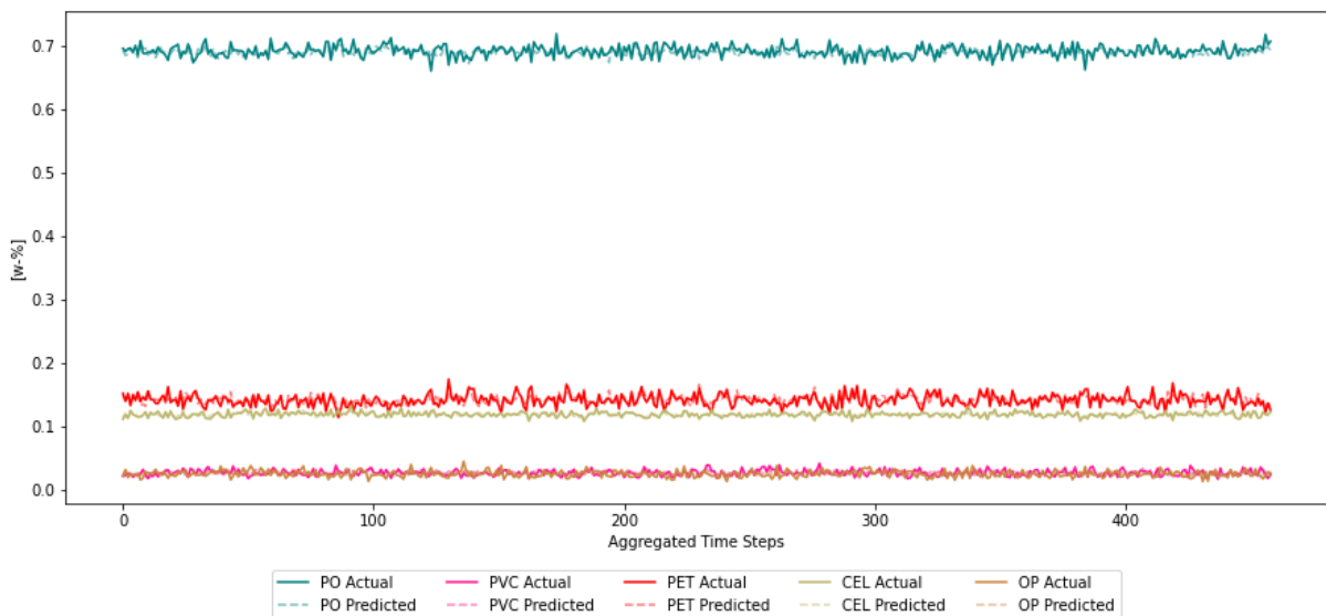
Figure 59: Weight shares on PO75C resulting from measured and predicted area flows, calculated with area densities obtained with OLS modelling and V9 pre-processing from PO75C and AA106, aggregation with 30 minutes per bin.
