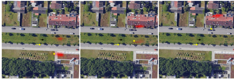
(a) Error distribution follows vehicle location distribution. Even though the semantic content may be very discriminative longitudinally, the longitudinal error is still larger than lateral, since the vehicle location is more uncertain longitudinally.
