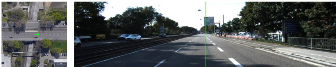
(a) Test2, sample 1217. Clearly the camera is in the middle, if not to the right of the middle lane. The ground truth is almost at the left lane marking. If we assume the average lane width to be 3.5 m, the lateral error on this image can be up to 1.75 m, which is extremely large for the fine-grained setting.
