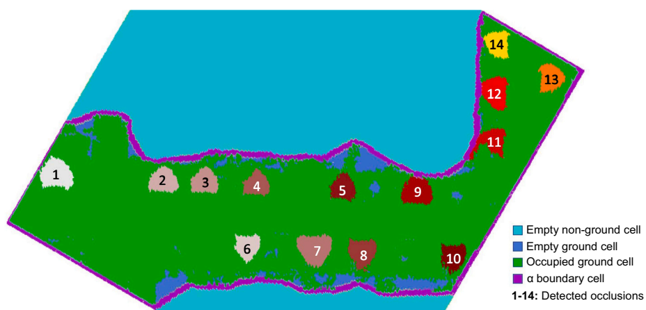
Fig. 15. The result of the occlusion detection (the scene is now street-aligned by rotating clockwise the scene from Fig. 14).
