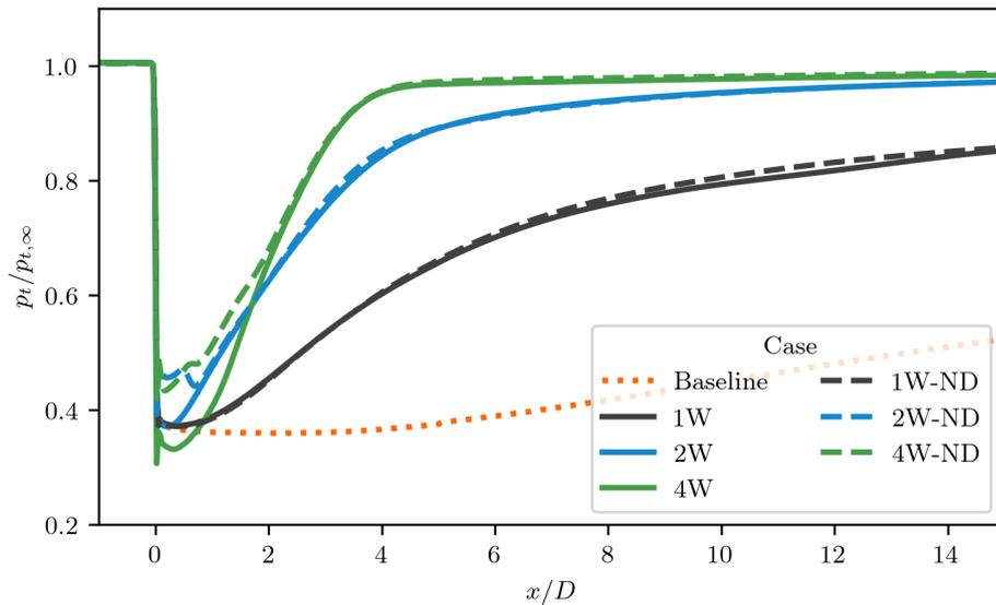
**Figure 13.** Total pressure distribution in the wake as a function of the streamwise coordinate,  $x/D$ , for all cases examined in this study. The total pressure is integrated within a box-shaped volume corresponding to the rotor’s projected area. Dashed and solid curves represent ABL-controlled setups with and without wing-induced drag, respectively. The dotted line represents the results for the system without ABL control.
