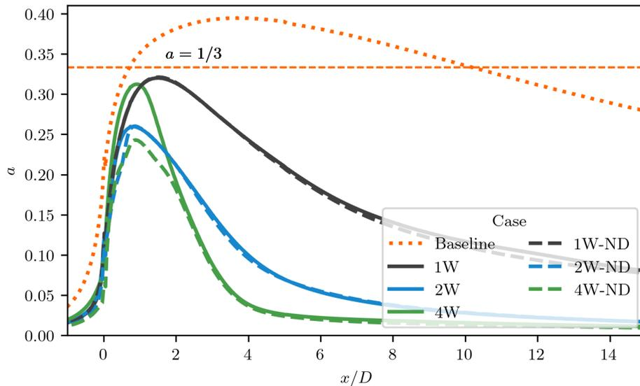
**Figure 15.** Effective induction factor in the wake for all cases examined in this study. Dashed lines represent systems without wing-induced drag, while solid lines represent systems with wing-induced drag. The dotted line corresponds to the system without ABL control, with the dashed orange line indicating the  $a = 1/3$  plateau, corresponding to the Betz limit.
