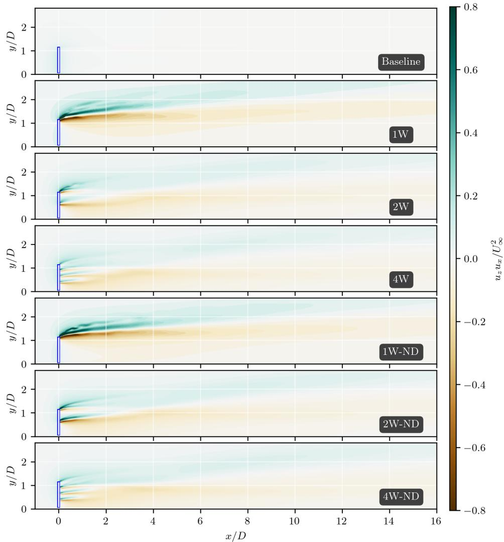
**Figure 12.** Crosswind and streamwise velocity products at a plane on the left-hand side of the disk actuator model (represented as a white box) at  $z/D = 0.5$ .
