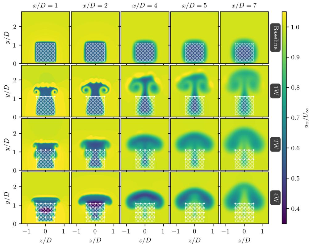
**Figure 7.** This figure extends the results shown in Fig. 6, accounting for the effects of the wing’s induced drag. Each panel shows the streamwise-colored wake behind the multirotor system (the rotor’s projected area represented by the hatched white region) at different downwind locations,  $x/D$ . Underneath the top baseline row, each row shows, from top to bottom, results for the ABL-controlled system with 1, 2, and 4 wings, respectively (represented by dotted white line segments).
