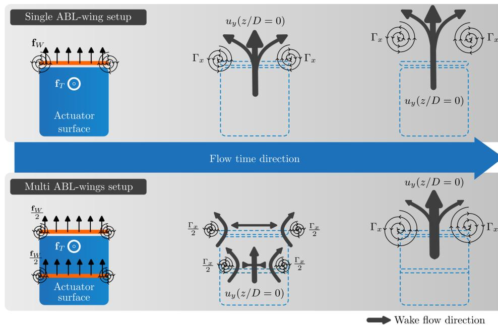
**Figure 10.** Schematic diagram illustrating the mechanisms driving upward advection in the wake. Setups with a single wing (represented by orange line segments) move wing-tip vortices farther up into the atmosphere. In contrast, setups with multiple wings elevate the wing-tip vortices more slowly but more efficiently transport low-momentum flow upward.
