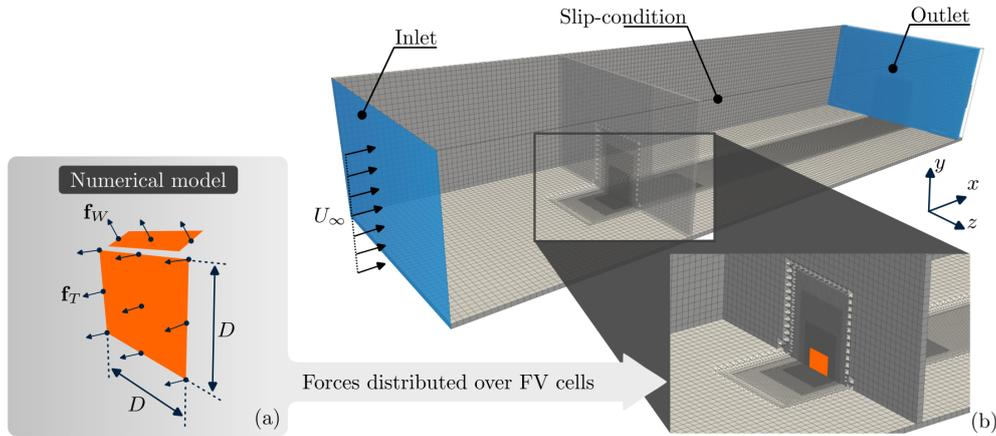
**Figure 3.** Panel (a) shows details of the numerical model based on momentum theory; panel (b) shows details of the computational domain with the actuator forces modeled as momentum sources. The computational domain is highlighted at the top.
