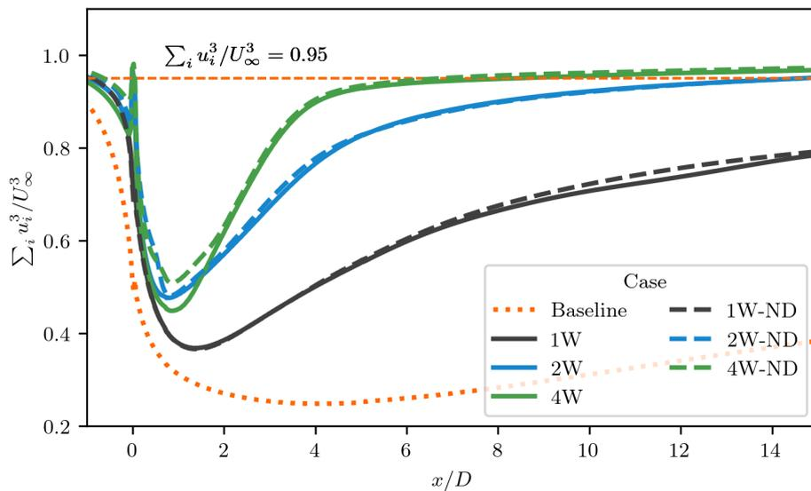
**Figure 14.** Cubed velocity for all cases examined in this study. Dashed lines represent systems without wing-induced drag, while solid lines represent systems with wing-induced drag. The dotted line corresponds to the system without ABL control, with the dashed orange line indicating the 0.95 recovery plateau for reference.
