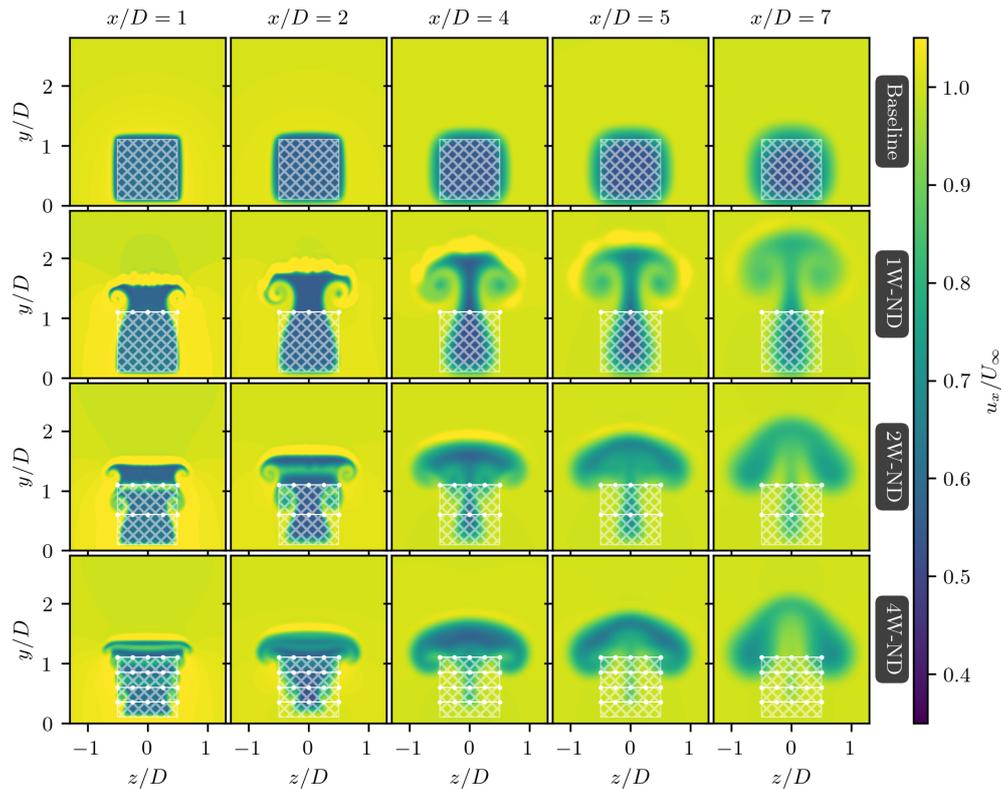
**Figure 6.** Streamwise velocity contours at various downstream locations,  $x/D$ , behind the multirotor system (with the rotor's projected area shown as the hatched white region). The top row shows the baseline case without ABL-control devices, while the subsequent rows present cases with 1, 2, and 4 wings, respectively (wings indicated by dotted white lines). The effects of the wings' induced drag are excluded from these simulations.
