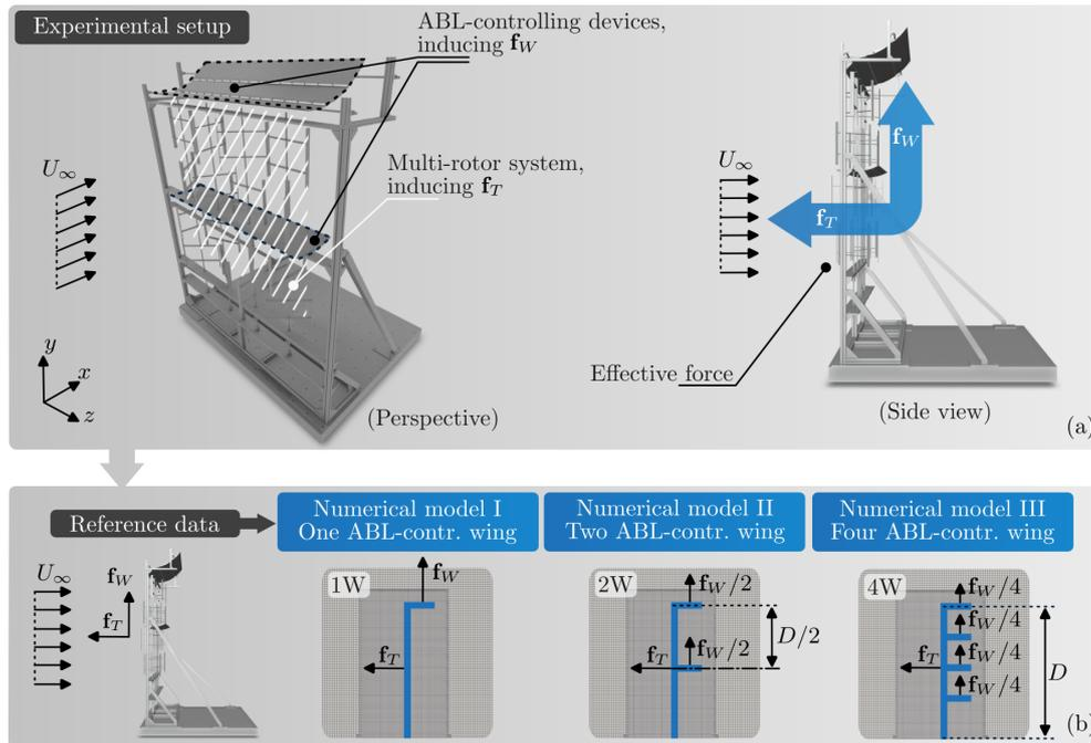
**Figure 2.** Panel (a) provides an overview of the reference experimental setup, while panel (b) presents the corresponding numerical model based on momentum theory. In the experimental setup, the thrust force vector of the multirotor system,  $f_T$ , and the effective aerodynamic force of the ABL-control system,  $f_W$ , are measured. In the numerical model, these forces are distributed homogeneously in a cell-weighted fashion to replicate the experimental conditions.
