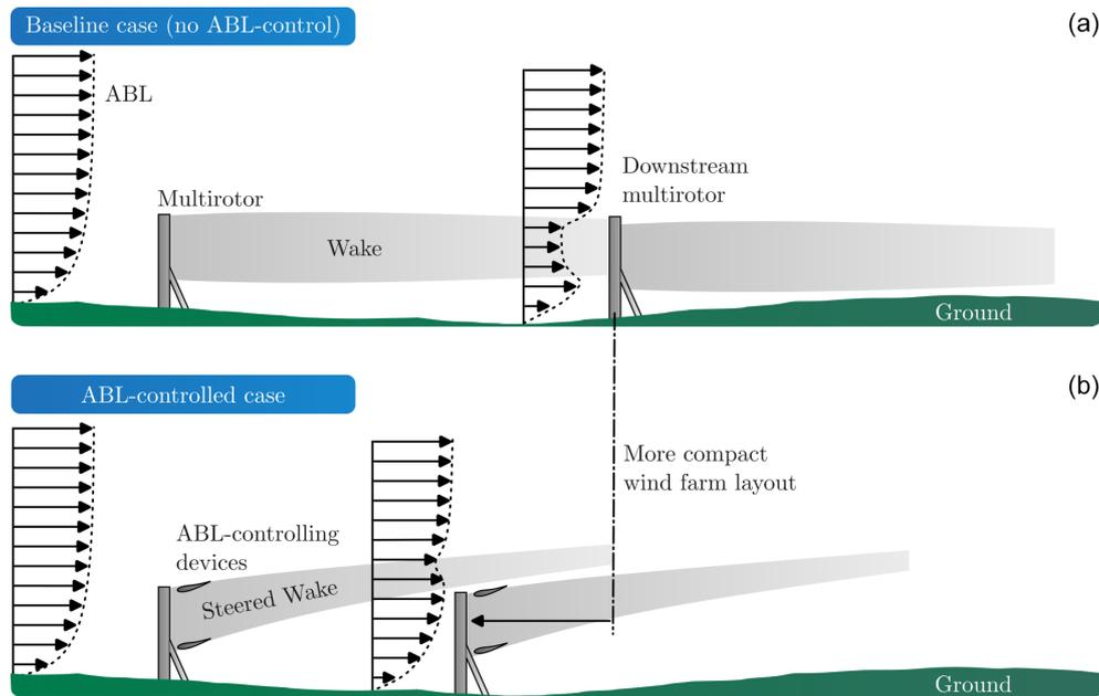
**Figure 1.** The figure provides a schematic representation of the wake generated by a multirotor system, shown before (a) and after (b) the implementation of ABL-control systems. The ABL control directs the wake upward into the atmosphere, enhancing vertical momentum flux and accelerating wake recovery. This mechanism allows ABL-controlled wind farms to achieve higher power output per unit of land or sea area, facilitating a more compact wind farm design.
