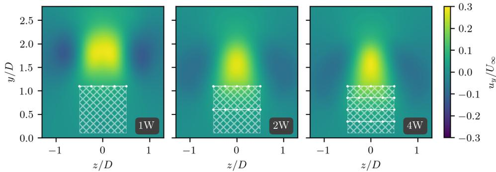
**Figure 9.** Vertical velocity  $u_y/U_\infty$  in ABL-controlled setups. The hatched white region represents the rotor’s projected area, and the dotted white lines depict the ABL-control devices. This figure confirms the behavior described by Eq. (10), showing maximum  $u_y$  at the  $z/D = 0$  plane.
