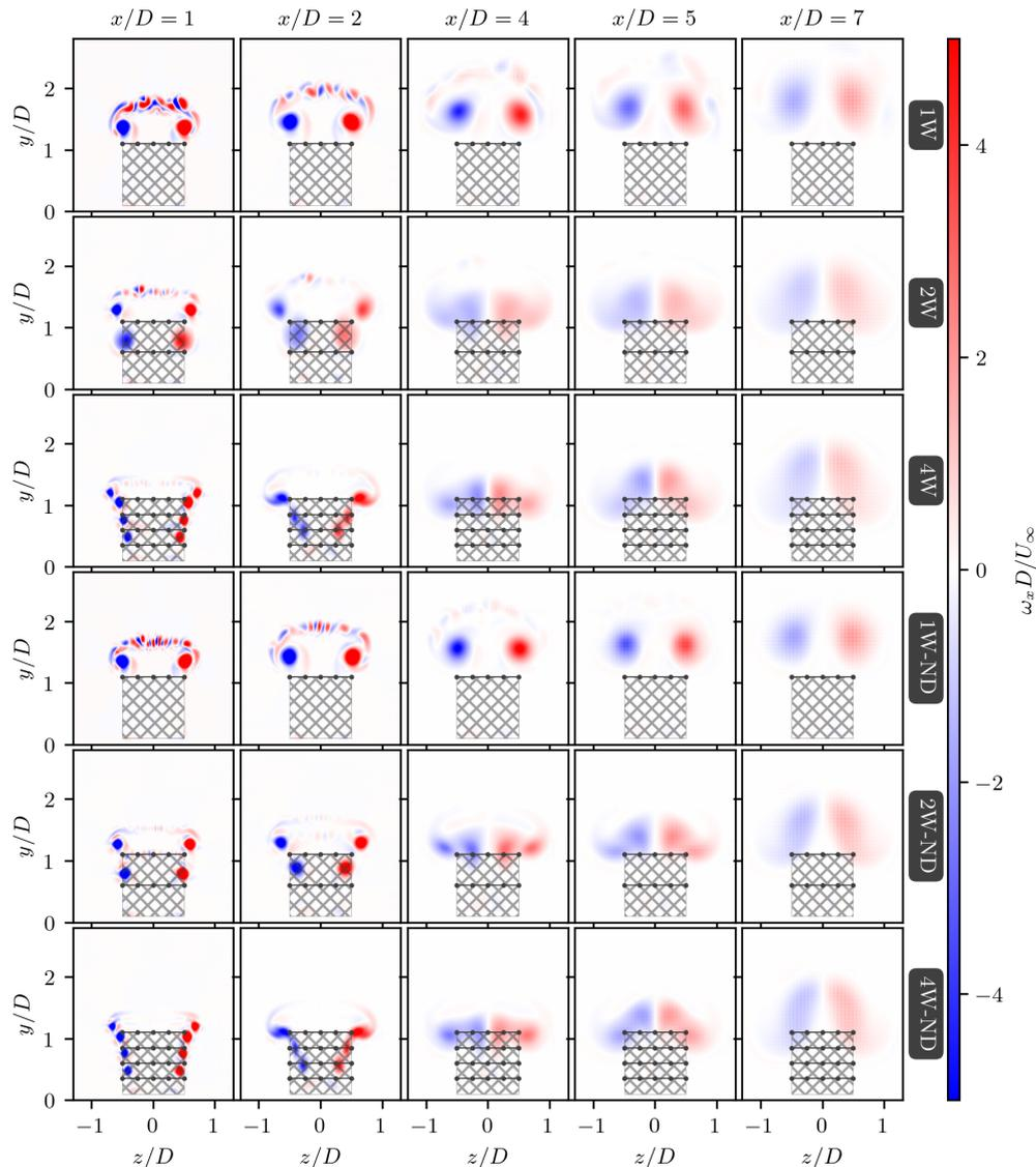
**Figure 8.** Streamwise vorticity contours highlighting the wing-tip vortices generated by different ABL-control configurations. From top to bottom, rows represent results for 1, 2, and 4 ABL-control wings with (first–third rows) and without (fourth–sixth rows) induced drag (depicted as dotted black line segments), respectively.
