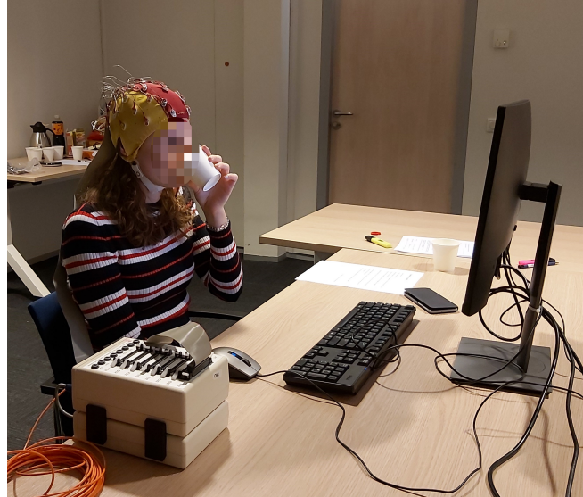
Figure 2.4: Experimental setup: participant seated in front of computer screen, wearing a 32-channel EEG-cap with electrodes placed according to the 10-20 system
