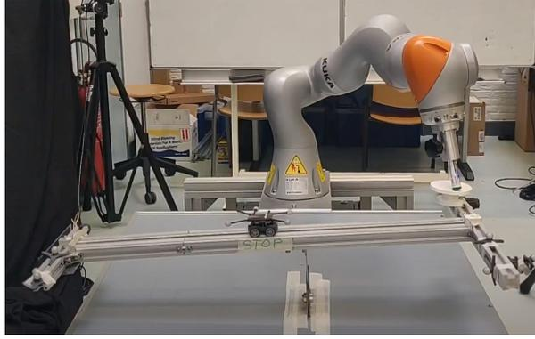
**Figure 5-3:** Modified environment to test state space policy: Balancing the car by pushing the lever on the opposite side.
