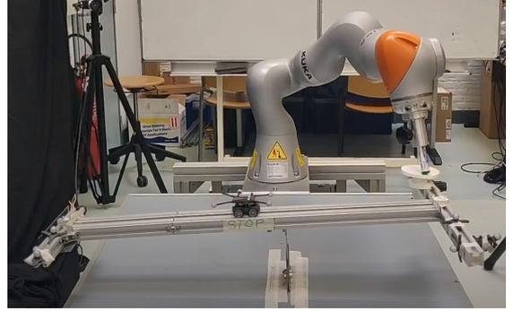
Fig. 3: Modified environment to test state space policy: Balancing the car by pushing the lever on the opposite side.
