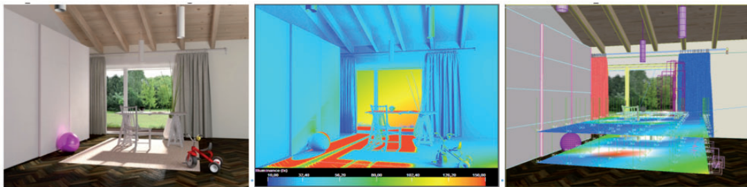
Figure 1 The leftmost image shows a scene, the middle image is a false colour representation of the illuminance over all surfaces of a scene, the right image is a false colour representation of the illuminance over planar cross-sections in the space (available in colour in online version)
