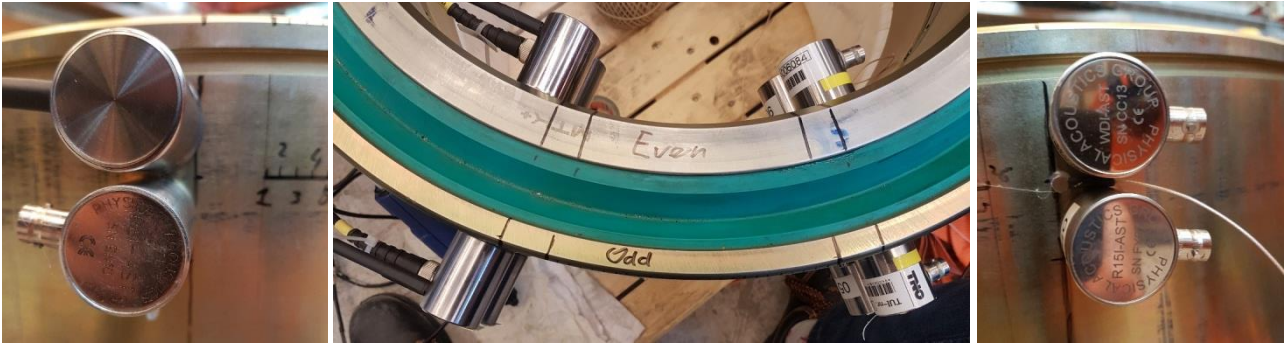
Figure 2: The experimental set-up: a top view of the instrumented bearing (middle), R3I-AST and R6I-AST type sensors (left), and WDI-AST, VS600-Z2 and R15I-AST type sensors (right).
