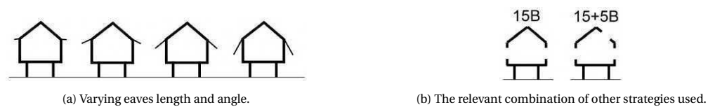
Figure 5.9: Varying eaves length and angle on air velocity with relevant combinations of other strategies.
