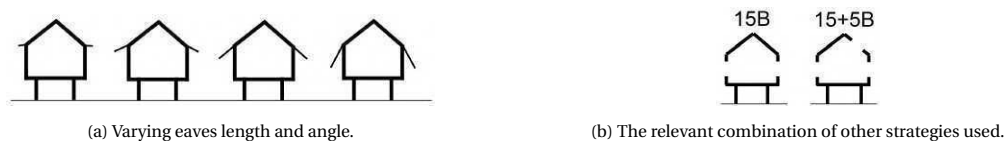
Figure 5.30: Varying eaves length and angle on air velocity with relevant combinations of other strategies.
