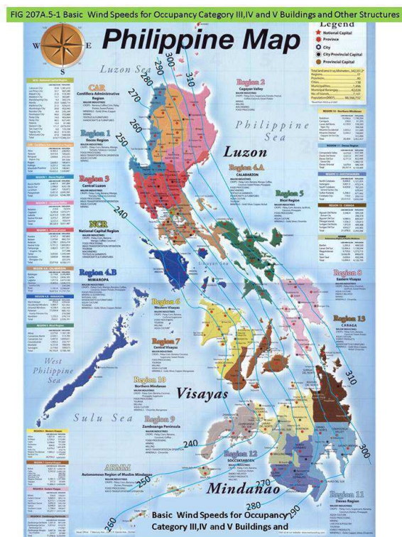
Figure A.2: Building code (NBCP) minimum wind speed requirements per area in the Philippines.
