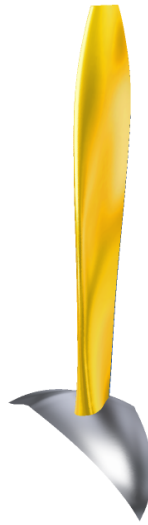
Figure 9.26: Visualisation of the XRPOP propeller used in the validation of the BEM and RANS tools
