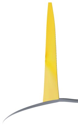
Figure 9.50: XPROP propeller with (small) curved fairing aft of the spinner
