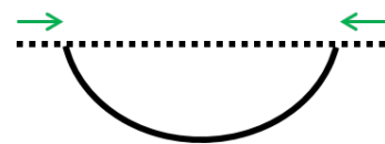
Figure 1: Visualisation of implying a transversal curvature by moving the boundaries towards each other. Dotted line indicates the flat configuration. Solid line indicates curved configuration.
