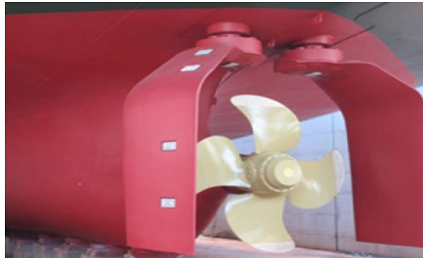
Figure 2.14: A gate rudder installed on the Shigenobu. From [10].
