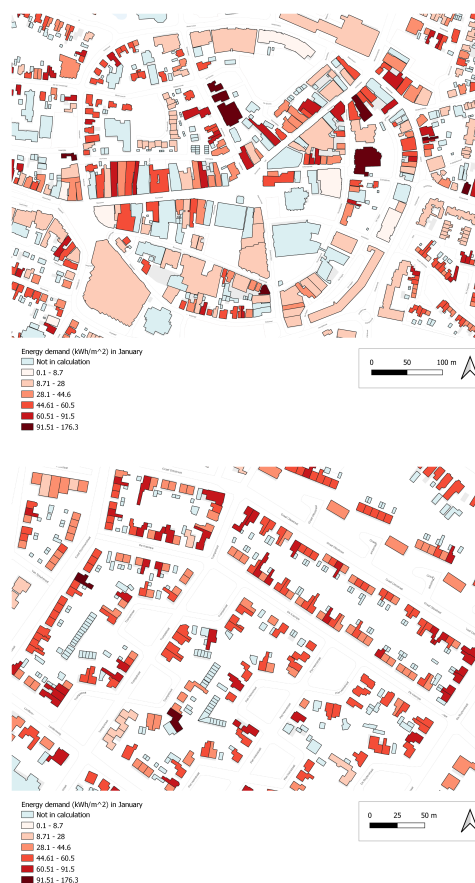
Figure 13. Energy demand (kWh) in the month January in the center (top) and a residential area (bottom) in Rijssen.
