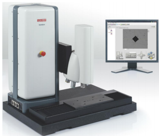
FIGURE 3.15: Durascan70 micro-hardness testing machine
