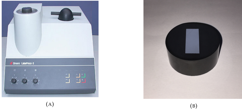
FIGURE 3.8: (A) Hot mounting press and (B) Sample mounted with conductive thermoplastic resin
