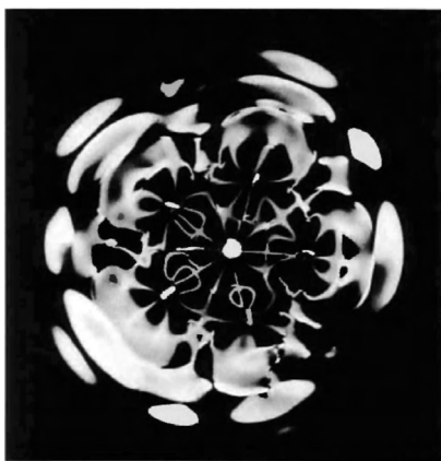
Figure 12. 44 A layer of glycerin excited by the oscillation of a membrane. Figures can also be seen in the liquid. From Cymatics: A Study of Wave Phenomena and Vibration (Revised Edition 2001, p6), by Hans Jenny, 1967/2001, Basilius Presse (1967, original publisher) MACROmedia Publishing (2001, publisher revised edition).
