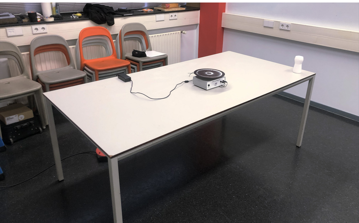
Figure 32. Setup 3: circular Chladni plate containing 240mm diameter; 1mm thickness; steel, salt was used for the particles.
