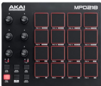
Figure 57: The Akai MPD218 MIDI controller used for all three concepts for slot selection and frequency and amplitude control
