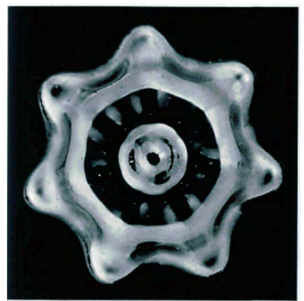
Figure 13. 118-123 [only showing 122] These photographs are of vibrating mercury drops. Since high surface tension causes mercury always to seek a spherical form, the drop does not disintegrate under the action of vibration. Instead the vibration becomes visible as a change of form. These pictures thus show true spatial configurations as seen from above. [...] From Cymatics: A Study of Wave Phenomena and Vibration (Revised Edition 2001, p6), by Hans Jenny, 1967/2001, Basilius Presse (1967, original publisher) MACROmedia Publishing (2001, publisher revised edition).
