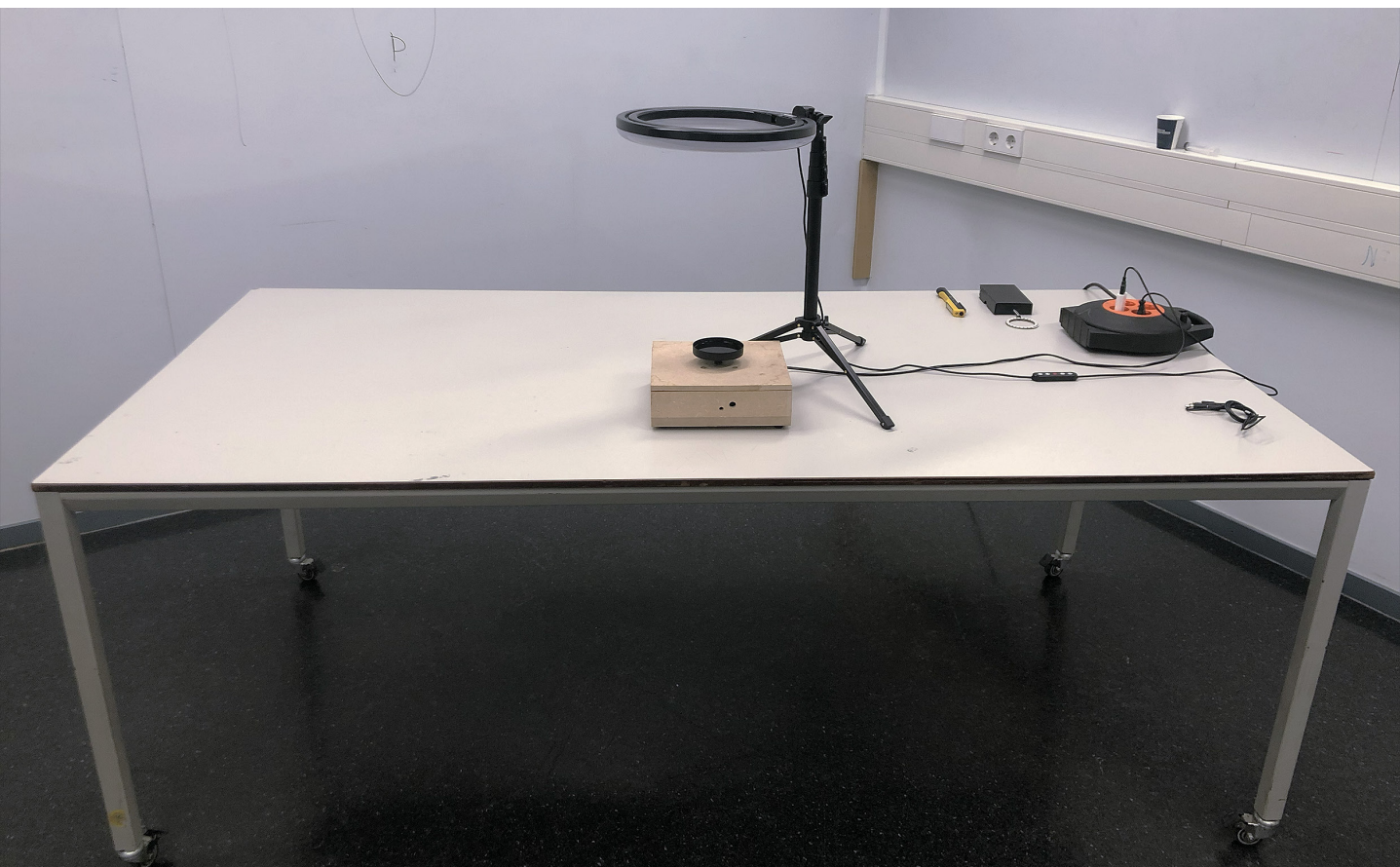
Figure 30. Setup 1: water cymatics setup containing 88mm diameter petridish; painted mat black, filled with water. Lighted with a MOMO RGB LED ring
