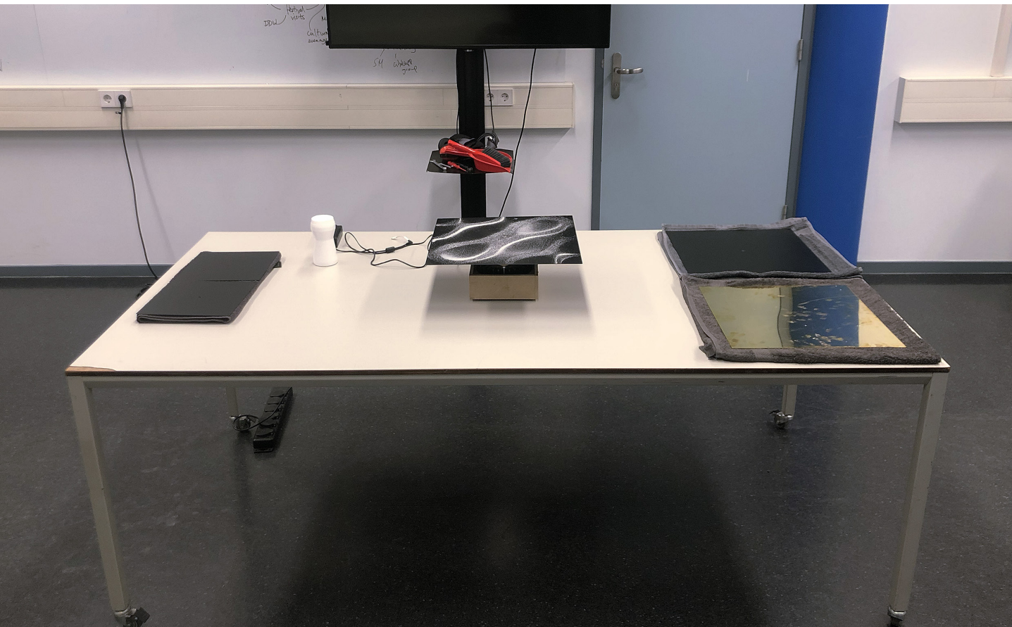
Figure 31. Setup 2: squared Chladni plate. Five different squared metal plates were tested, including 400mm square; 2mm thickness; steel, 400mm square; 1mm thickness; aluminium, 400mm square; 2mm thickness; brass; 240mm square; 2mm thickness; steel, 240mm; 1mm thickness aluminium, salt was used for the particles.
