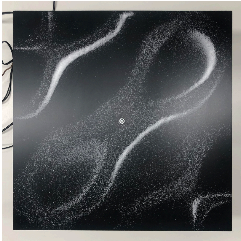
Figure 22. Chladni pattern at 91 Hz, steel 400mm square, 2mm thickness
