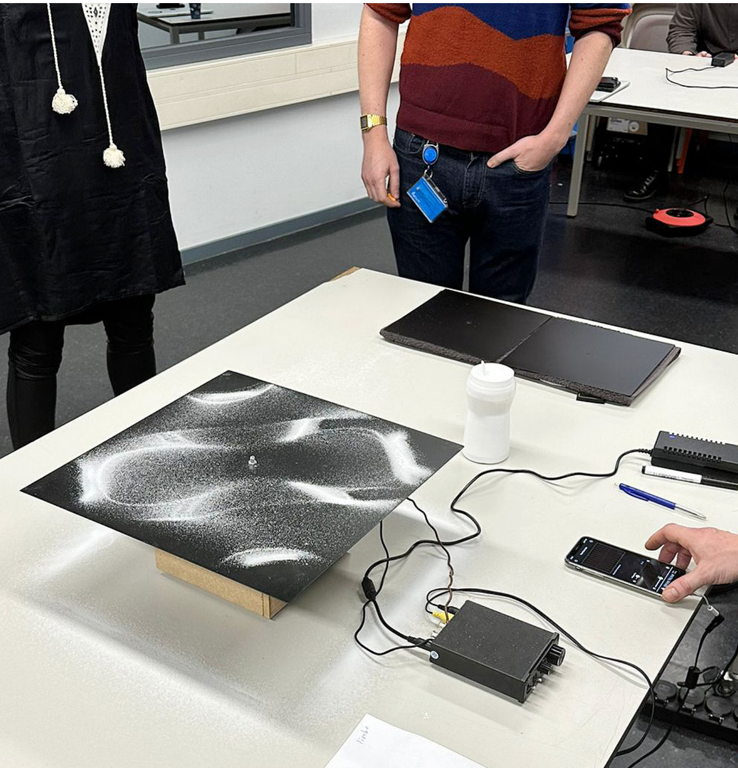
Figure 33. Session 0 demonstration of setup 2 squared Chladni plate with IDE faculty members.
