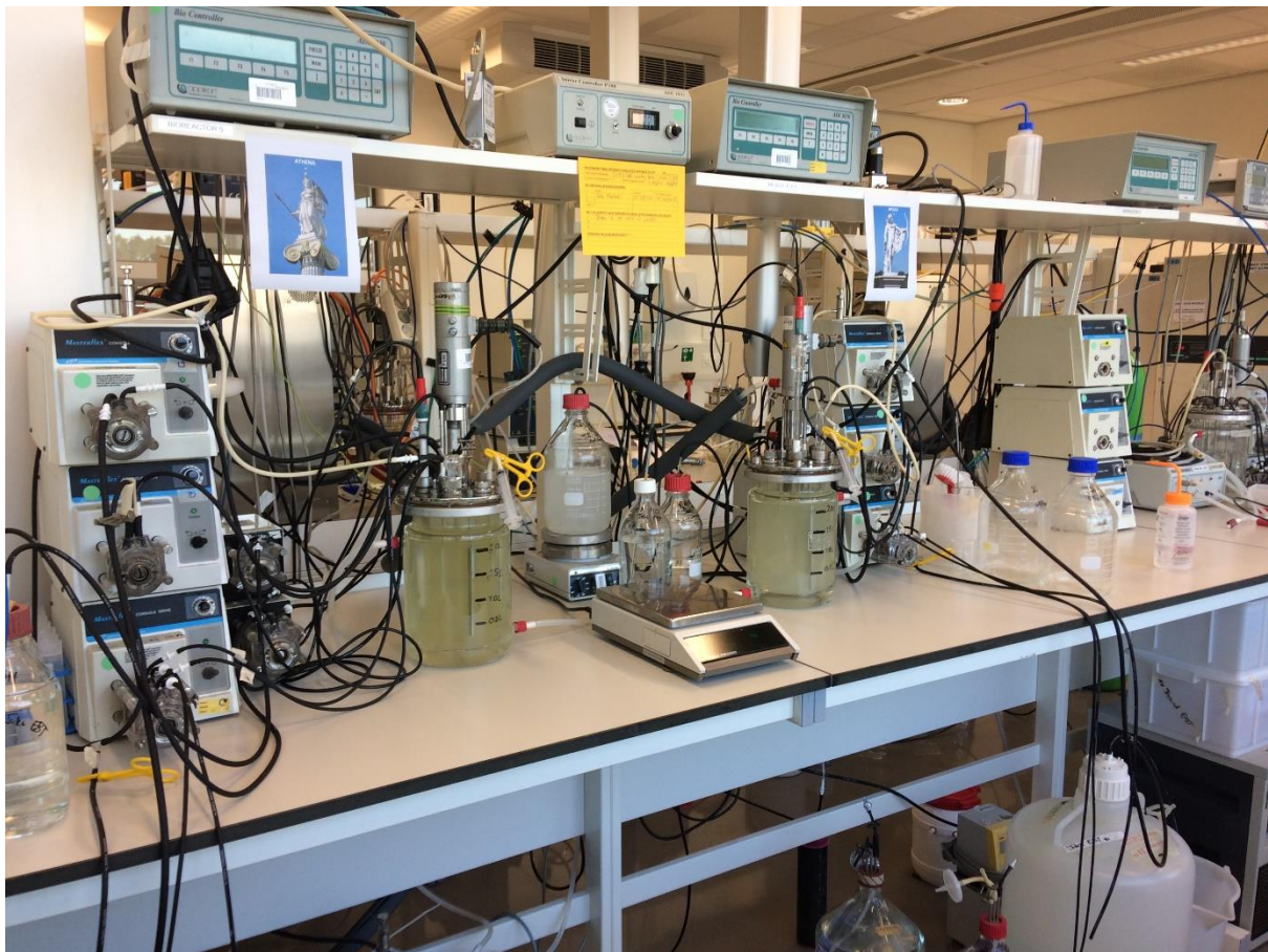
Figure 1.9: Typical bioreactor enrichment set-ups used in this thesis. Here, the bioreactors ran in parallel to study xylose and glucose fermentations in SBR mode are shown, ran in September/October 2017.
