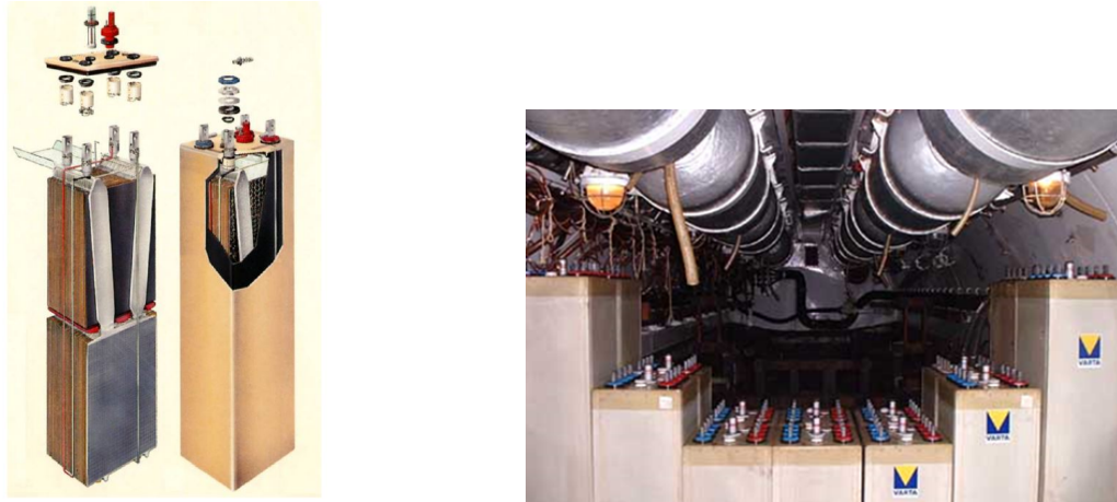
(a) Construction of submarine lead-acid cell [28] (b) Battery compartment Dolfijn-class submarine
