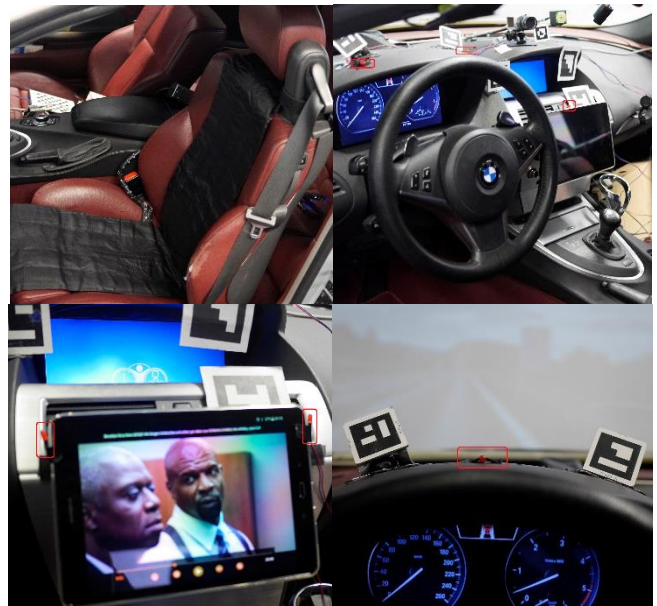
Fig. 1. Interior of the driving simulator. The top left figure shows the vibration mat in the driver seat. In the top right figure the LEDs are configured in the call-session, namely two red LEDs on the dashboard beyond the steering wheel, and one above the tablet (indicated by red rectangles). The tablet can be seen on the center console and in the bottom left figure. The bottom right shows the instrument cluster and LED on the dashboard above the steering wheel.
