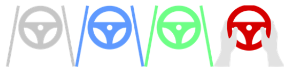
Fig. 2. Icons indicating the automation status (gray = disabled; blue = available; green = active; red = take-over).
