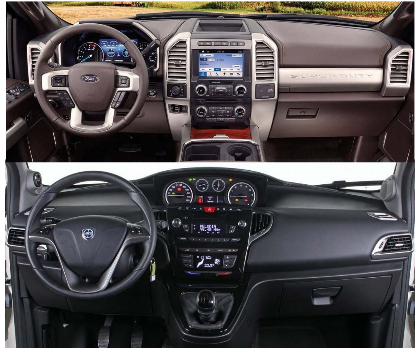
Figure 5 - Two vastly different vehicular HMI designs - Ford F250 (2018) on top, Lancia Ypsilon (2012) on the bottom
