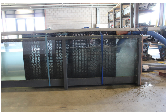
(a) Perforated boxes to stabilise the water flow at the entrance of the flume
