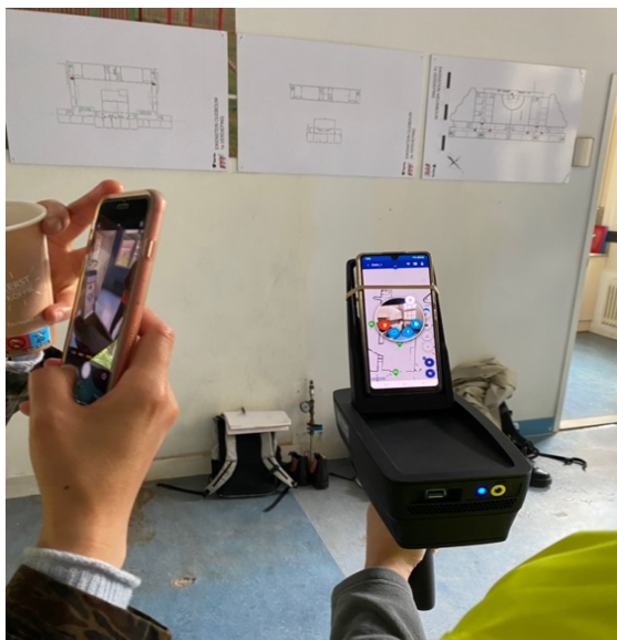
Figure 10. Equipment for pre-demolition audit
