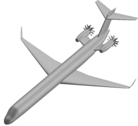
Figure 1.2: Typical aircraft configuration with rear-mounted contra-rotating open rotor engines. Reproduced from [10].
