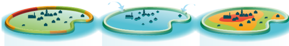
Figure 2.9: The probability of failure times the consequence, gives the risk shown in the last drawing, from (Rijkswaterstaat Projectbureau VNK, 2014). In the left figure the probabilities of failure are indicated by color, in which red stands for large probability, orange a moderate probability and green for small probability. In the middle figure the effect of a flooding is shown. The right figure indicates the combined effect of probability and effect and can be expressed as economical loss or loss of life or a combination of both.
