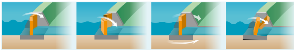
Figure 2.11: Failure mechanisms for a (moving) structure (from left to right): overtopping and/or overflow, not closing/not opening of the structure, water flow under or past the structure and structural failure, from (Rijkswaterstaat Projectbureau VNK, 2014).
