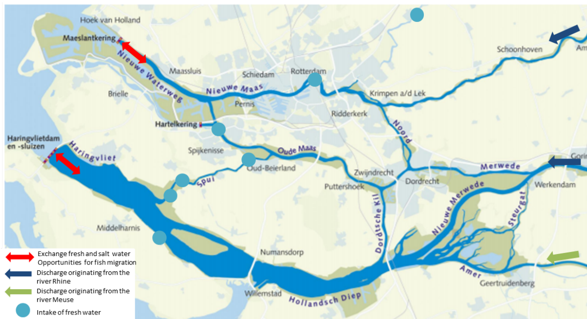
Figure 1.2: The incoming river flows from both the Rhine and Meuse. The exchange of fresh and sea water at the Nieuwe Waterweg and Haringvliet. The discharge distribution between the Haringvliet and Nieuwe Waterweg is regulated by multiple structures upstream and by the Haringvliet Sluices. The salt and fresh water mix at the mouth of the Nieuwe Waterweg. The location of mixture is expected to be dependent on the Rhine discharge, wind velocity and direction, water level at sea and the flow area at the Haringvliet sluices.
