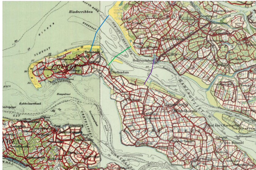
Figure A.2: Three possible locations for the closure of the Haringvliet, from Ferguson (1971).
