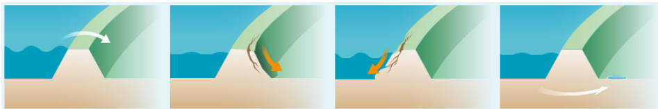
Figure 2.12: Failure mechanisms for dikes (from left to right): overtopping and/or overflow, instability of the dike, erosion of the revetment and piping, from (Rijkswaterstaat Projectbureau VNK, 2014).
