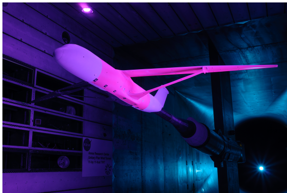
(a) An aircraft model coated with PSP (pink) mounted in the wind tunnel at NASA's Ames Research Center, duplicated from www.nasa.gov
