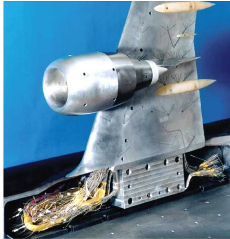
Figure 1.3: Wind tunnel model of an aircraft wing, showing the bunch of tubes connecting surface pressure taps to transducers
