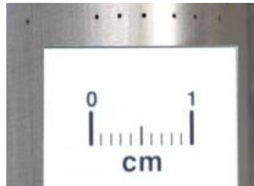
(b) Wind tunnel model showing the pressure taps on the surface along with a scale for reference, adapted from www.nasa.gov
