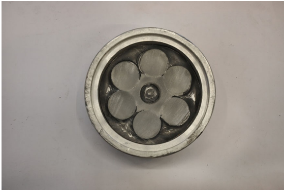
Fig. 7 The aluminium cap with the inlayed lead sheet and a section of the glass bundle
