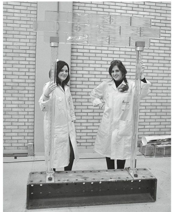
Fig. 2 Realized 1.5 m long prototypes of the bundled glass column
