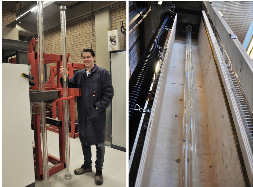
Fig. 15 Right Prototypes of the B_2 series using the spliced lamination principle in a spiral configuration, seen on the left
