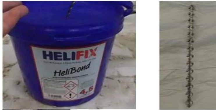
Figure 2-13: Repair mortar and twisted steel bar (Licciardello & Esposito, 2019)
