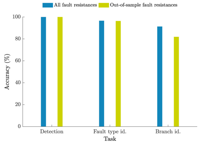
Fig. 10. Comparison of the average accuracy of the three tasks between all studied fault resistances between 3 and 500 \Omega and the out-of-sample fault resistances.
