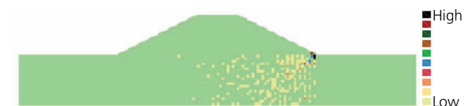
Figure 11. Locations of the points with maximum local velocity from 500 realisations ( COV_k = 1.0 and \xi = 20 )
