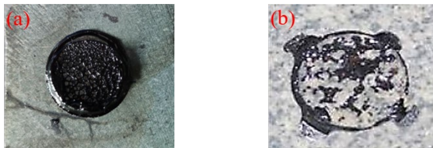
Figure 11. Examples of Bond strength Testing Failure Modes for bitumen-aggregate system: (a) Failure within the binder, (b) Failure at the binder/substrate interface.
