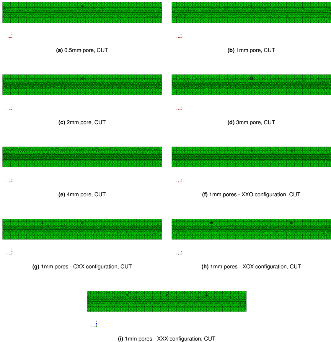
Figure 4.5: Sections displaying the pores configuration - Mesh 1
