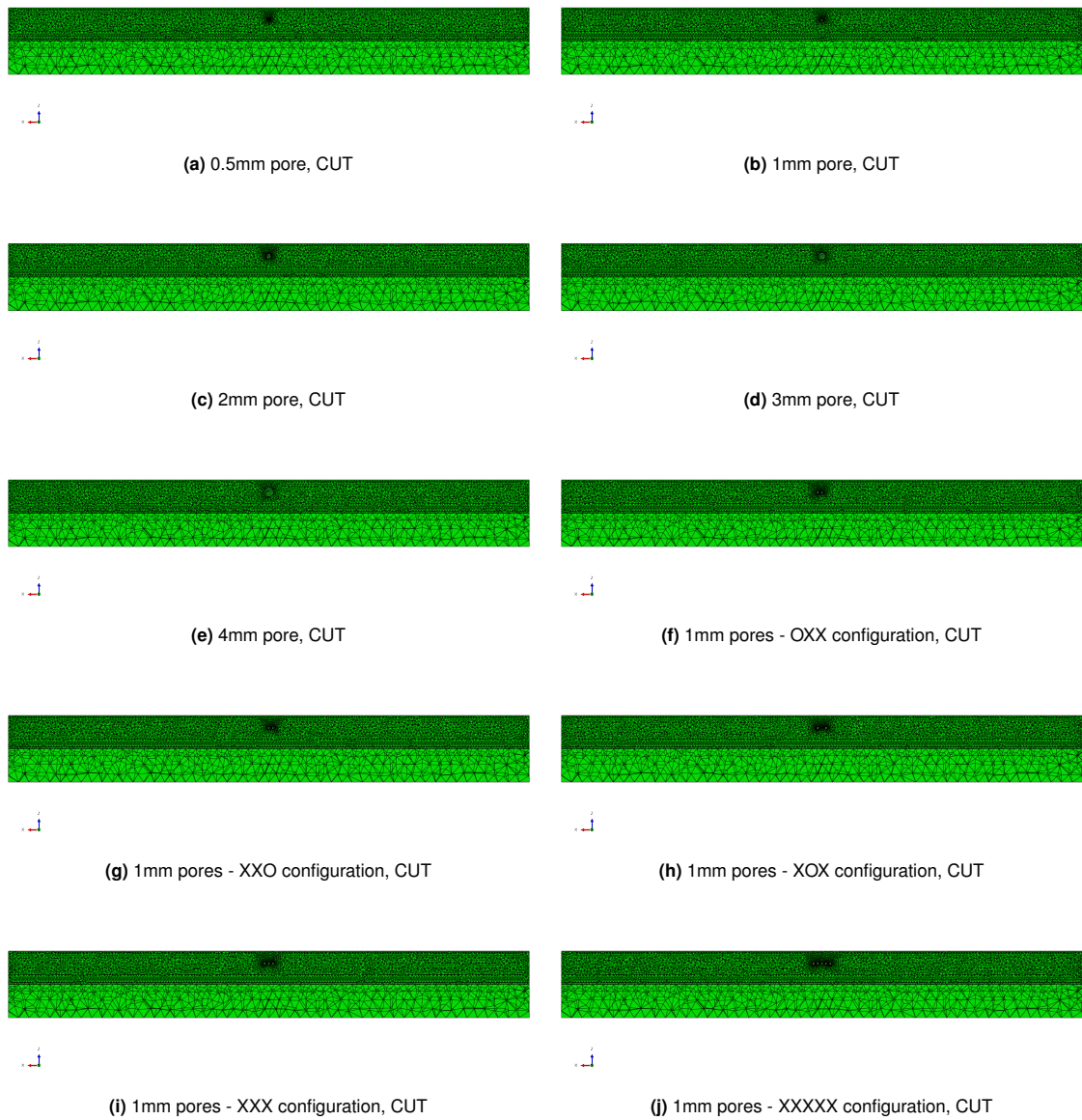
Figure 4.7: Sections displaying the pores configuration - Mesh 2
