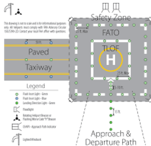
Figure 15.1: Heliport design standards [26]
