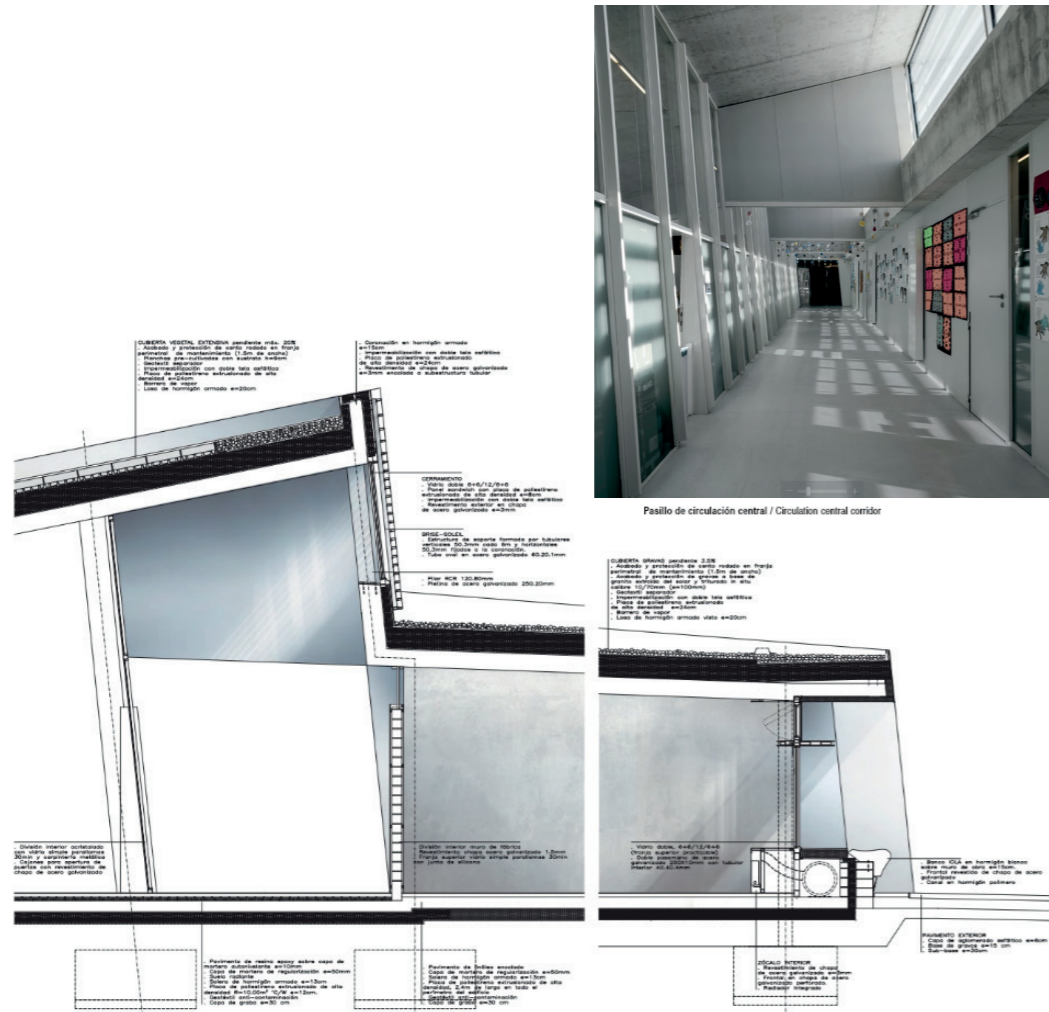
Figure 5.024 – Detail Sections and photograph through internal street, Sun School, RCR architects (2014) • Source: El Croquis
