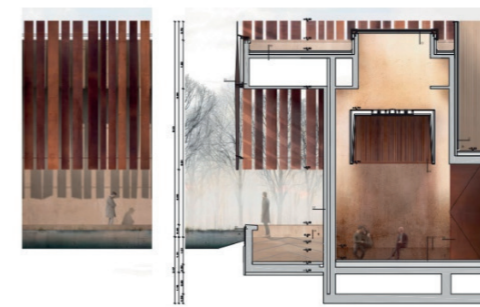
Figure 5.033 – Detail section and photograph, waiting room and verandah, Hofheide crematorium, RCR architects (2015) • Source: El Croquis
