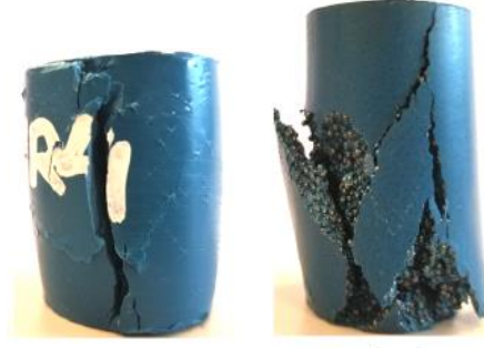
Figure 4: Typical failure modes for resin (left) and steel-reinforced resin (right) specimens.
