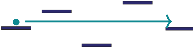
Figure 6.2: Cartoon of the VRH model. Here the electron does not need to move to the next nearest site, but may optimize the hopping distance r for a minimal \Delta E .
