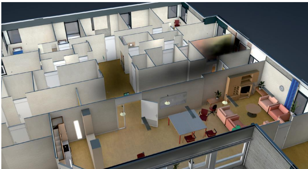
Figure 3.2 Visualization of psychiatric institution. Shown is the development of the fire and smoke spreading out of the patient room (Dutch Safety Board, 2012).
