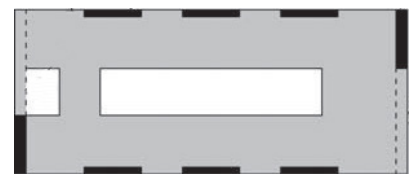
Figure 27. collector members in x direction are needed to transfer y direction force to shear force.
