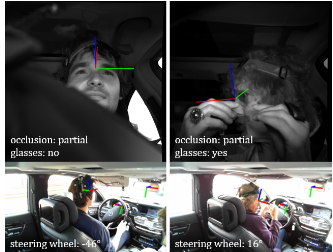
Fig. 1: DD-Pose provides precise 6 DOF head pose annotation for 330k stereo image pairs acquired in an in-car environment. The benchmark offers significant out-of-plane rotations and occlusions from naturalistic behavior introduced by complex driving scenarios. Annotations for partial and full occlusions are available for each high resolution driver camera image. An additional camera capturing the interior of the car allows for further multi-sensor driver analysis tasks.
