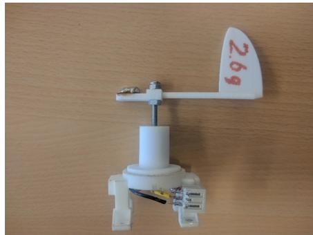
Figure 3.4: One of the wind vanes used to measure the angle of attack.
