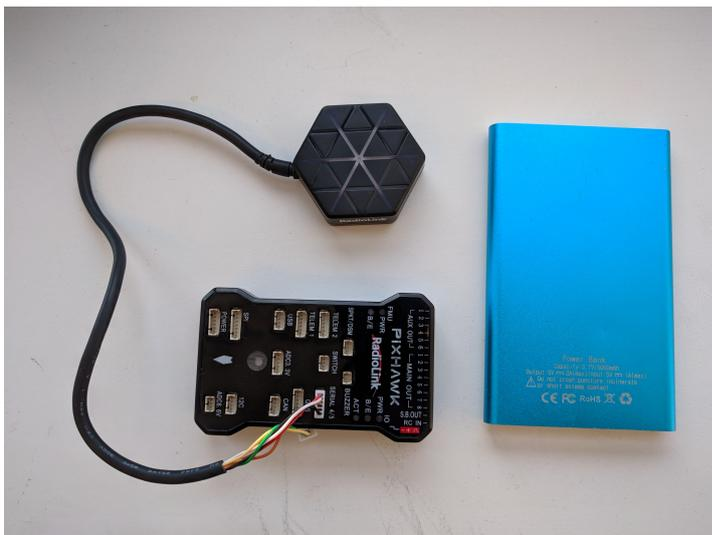
Figure 3.5: A Pixhawk and together with a gps module, these are powered by a power bank over usb.
