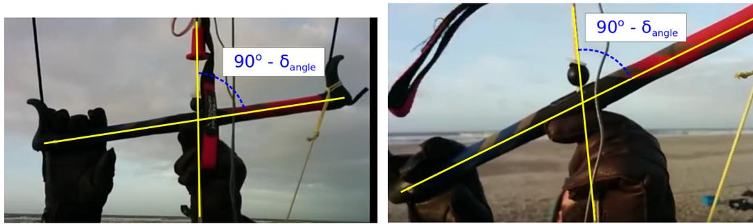
(a) The first setting of the stopperball allowed the pilot to steer the kites with a steering bar angle of  $8^\circ$ . (b) The second setting of the stopperball allowed the pilot to steer the kites with a steering bar angle of  $20^\circ$ .
