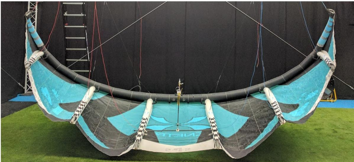
Figure 3.10: The test boom is attached to the kite by means of a boom normal to the test bar. This normal boom is attached where the red and blue steering lines on the most central struts are attached.
