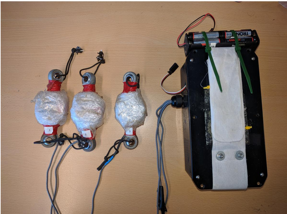
Figure A.1: The self made force measurement system consisting of three load cells and a blackbox with electronic devices and microcontrollers.
