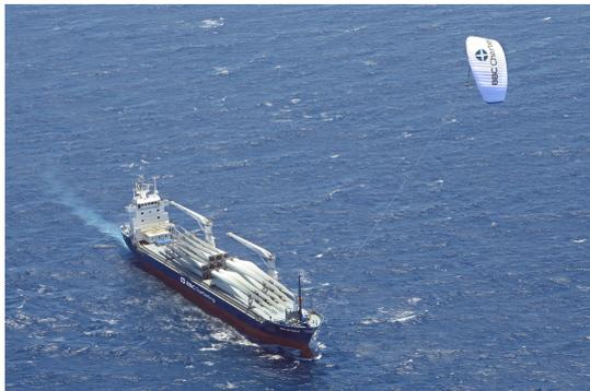
(a) The BBC Skysails with towing kite. The 132-m vessel utilizes kites of sizes up to 320 m<sup>2</sup>.source: [19]
