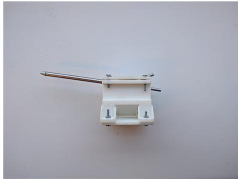
Figure 3.2: The pitot tube in it's mount to attach it to the measuring boom.
