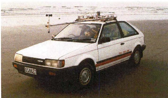
Figure 1.10: Photograph of the test rig mounted on the car. This first crude attempt to measure different aspects of the performance of kites proved to be good for initial testing but not for highly quantitative experiments. source: [21]
