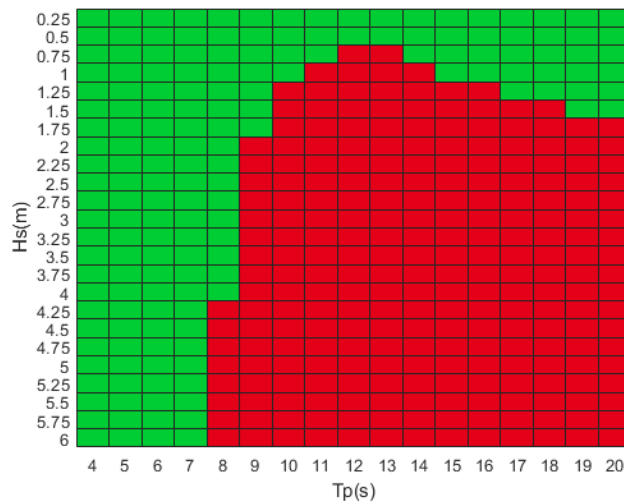
Figure D.1: The conditions at which the vessel does not exceed a roll angle of ten degrees
