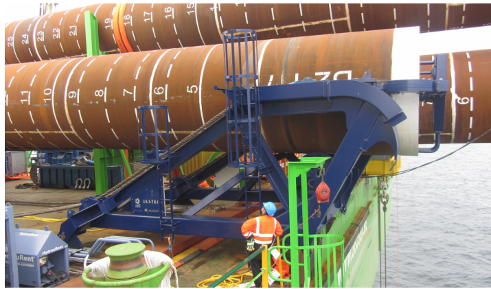
Figure 2.1: A monopile upending frame
