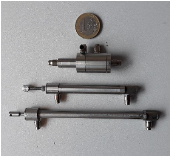
Figure 28: Photo of the prototype with a euro as a scale reference. From top to bottom; the booster, the hand cylinder, and the shoulder cylinder.
