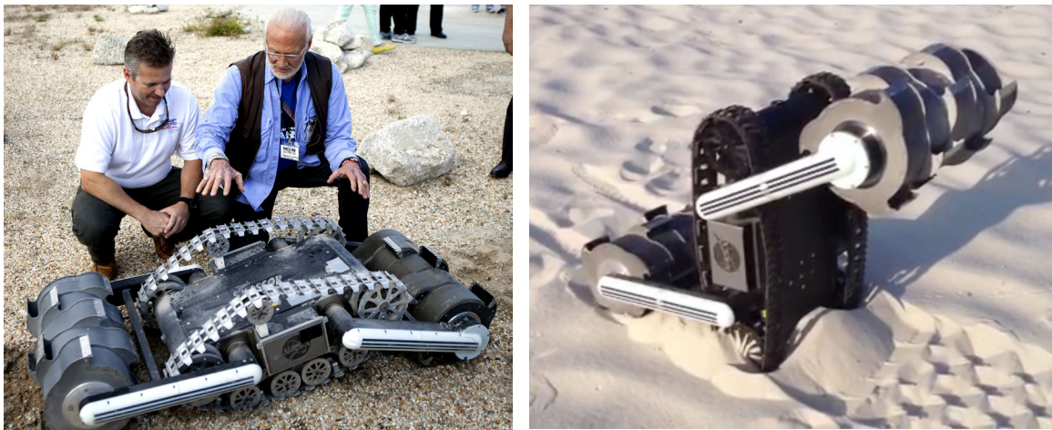
Figure 95. RASSOR prototypes. The size and principle of the excavations units are shown (Mueller, et. al., 2015).
