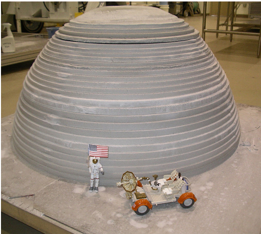
Figure 67. Prototype of a lunar habitat build with lunar regolith simulant using CC (Khoshnevis, et al., 2005).
