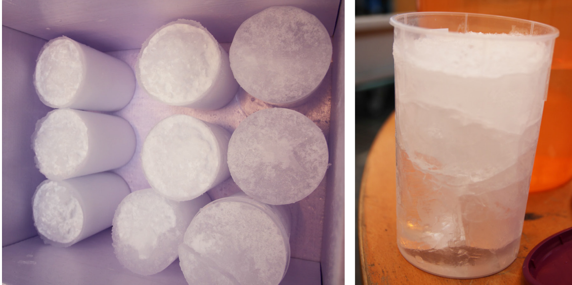
Figure 57. The picture on the left shows all the specimen from experiment C with the three specimens on the left being ice with a salinity of 15 ppt, the three in the middle ice with a 10 ppt salinity and the three specimens on the right being a 0 ppt salinity ice. This picture shows the difference in ice translucency. The picture on the right shows specimen C0.001, full of cracks even before demoulding.
