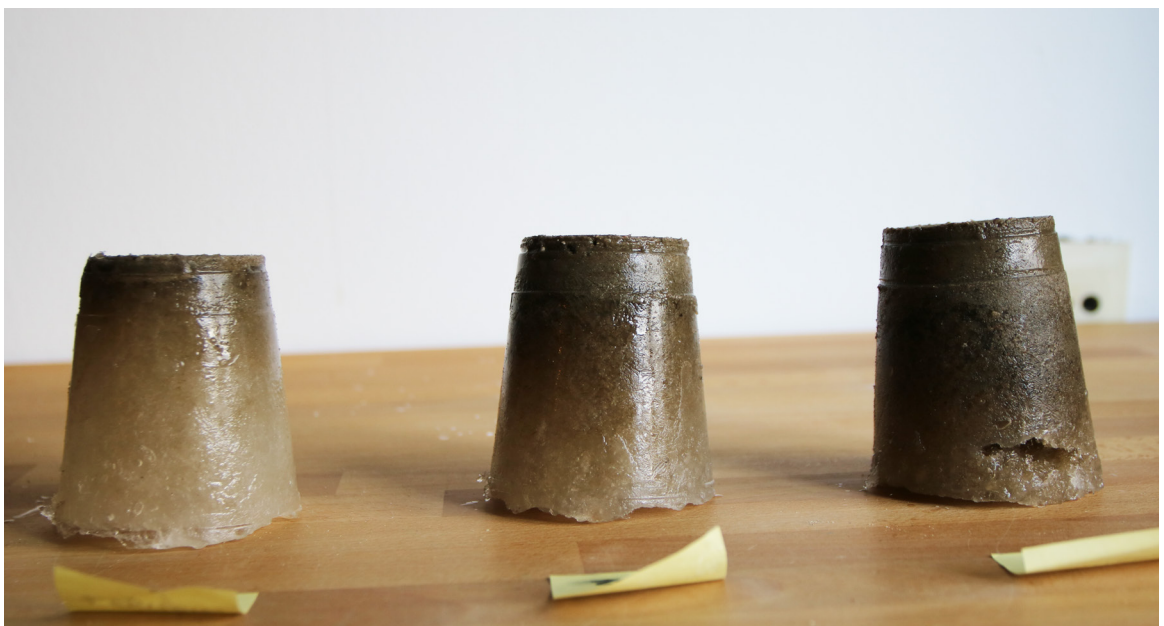
Figure 48. Experiment A. f.l.t.r Sample 006-008-010: Ice with different concentrations of sand – Sample 007-009-011: Ice with different concentrations of sand and 5gr of NaCl
