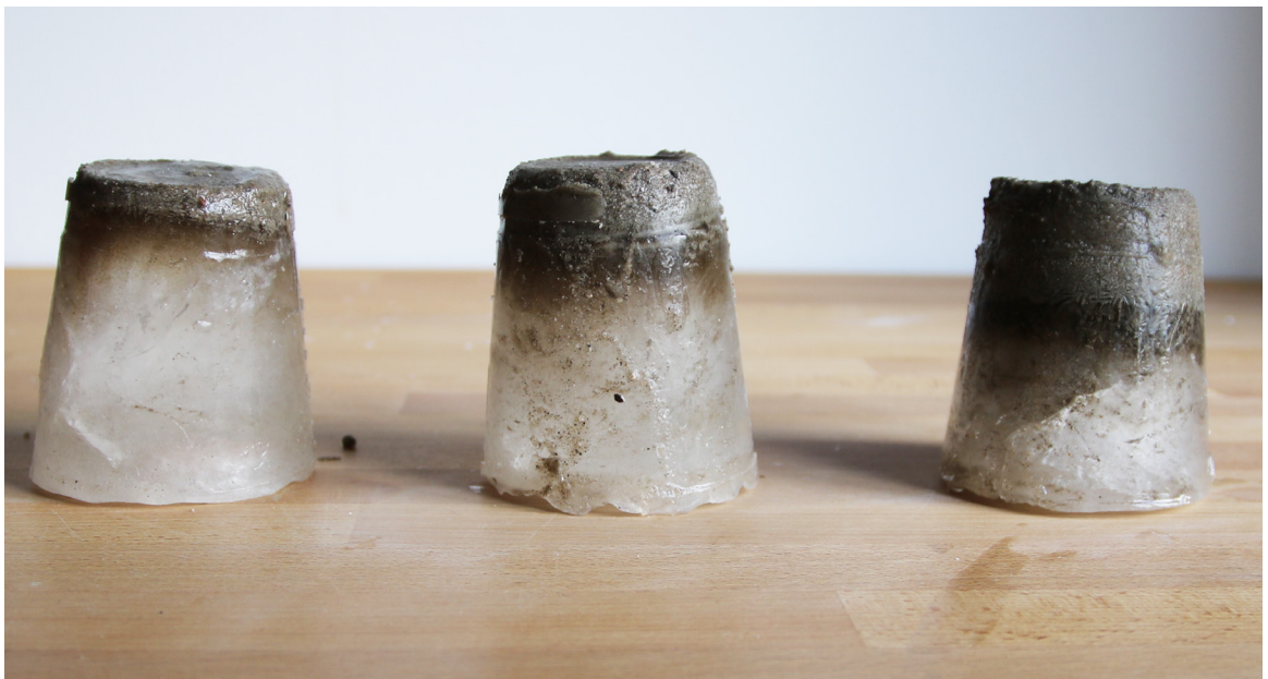
Figure 47. Experiment A. f.l.t.r Sample 003: Zero measurement – Sample 004: Plastic PP & HDPE – Sample 005: Plastic PP & HDPE and NaCl.
