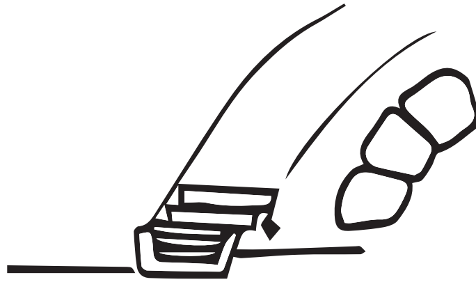
Figure 71. Building a dome out of water layers which freezes into ice requires a design solution for the cantilever part.
