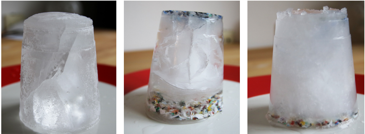
Figure 47. Experiment A. f.l.t.r Sample 003: Zero measurement – Sample 004: Plastic PP & HDPE – Sample 005: Plastic PP & HDPE and NaCl.
