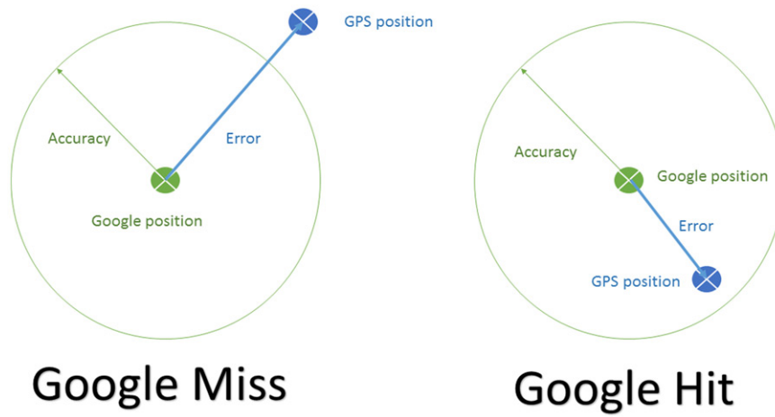
Figure 2. Description of what is considered a Google hit/miss. Google gives a radius of accuracy in meters where it is possible to find the device at a given time. Measuring the distance to the ground truth point (location provided by GPS device) we determine if the device was truly inside the circle. If it is, we call it a hit, otherwise it is a miss.
